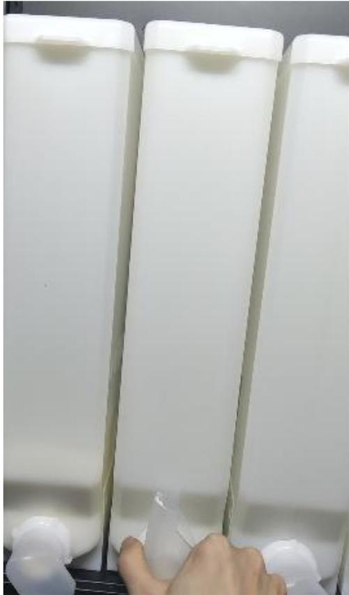
3) Open the cover on the canister top to add ingredient, there is a spiral on the cover where you can put drying agent to prevent the ingredient from getting wet.
