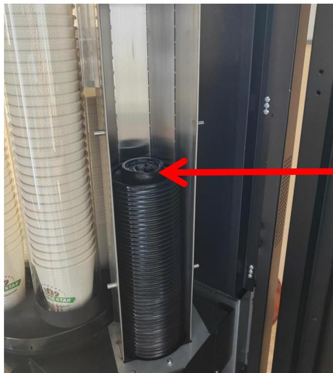
Make sure the protrusion side is up when placing the lids.
