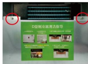
Note: When cleaning evaporator, please pay attention to not let the temperature probe touch the radiator and inner metal part of the evaporator. It should be fixed on the watercontaining plate to avoid affecting the cold storage temperature.
