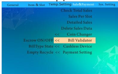
Press ▲2/▼8 to disable or enable Bill Escrow. If the machine needs bill change, the bill change switch must be turned on. Press "Enter" to save the setting.
