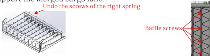
3. Disassemble the right spring and replace it with the right-handed spring. Remove the price tag of the right cargo lane and use the price tag of the left lane (for example, after the merger of 141 lane and 142 lane, the merged lane is 141).
