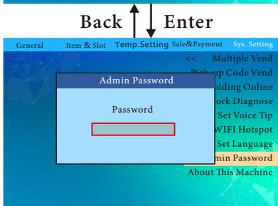
Press the keyboard to input the original password, then input the new password and retype the new password, press the "Enter" button to save the settings.
