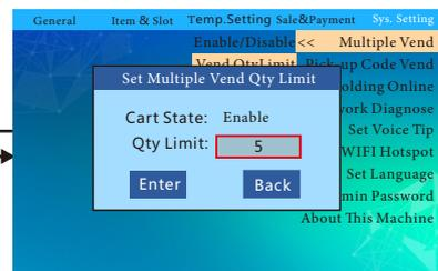
The shopping cart switch must be enabled before setting the number of shopping carts. The maximum number of shopping carts can be set to 5. After the setting is completed, press the "Enter" button to save the settings.
