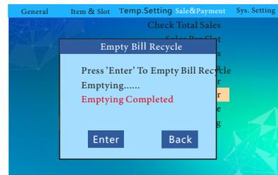
Press the "Enter" button to empty the Bill Recycle and press the "Back" button to return to the previous interface.
