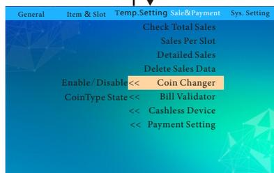
Press ▲2/▼8 to select to disable or enable coin change. If the machine needs coin change, the coin change switch must be turned on. Press "Enter" to save the settings.
