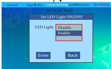
Press ▲ 2 / ▼ 8 in the keyboard to select Disable or Enable, select whether the lighting strip is on, press the "Enter" button to save the settings.
