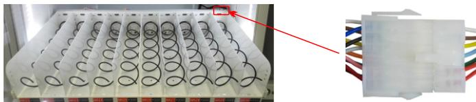
2. Unscrew the spring on the right side of the cargo lane to be merged, disassemble the middle baffle screw of the cargo lane to be merged (the plastic baffle can be pushed directly inward and removed) and remove the baffle. Note: the baffle fixed by rivets does not support the merged cargo lane.
