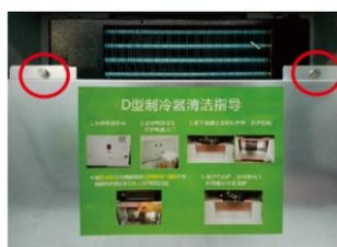
4. Remove baffle and insulating tin foil
