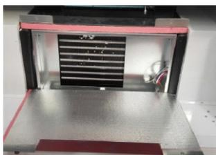
5. Clean up the dust with a nonmetallic soft brush the gap of the radiator.
