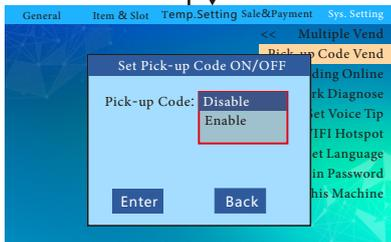
Press ▲ 2 / ▼ 8 in the keyboard to select to disable or enable the pick-up code switch, press the "Enter" button to save the settings.
