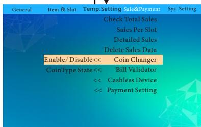
After the coin type is enabled, 14 digits (02-15) must be turned on (blue in the selection box is on, blank is off), press the Enter button to turn it on or off the Enables, press the 4/6 button to shift left and right. If the 00 bit enable is on, it means receiving 0.5 yuan coins, 01 bit enable is on, it means receiving 1 yuan coins, press the Back button to save and press the Back button to the previous interface after setting is completed.
