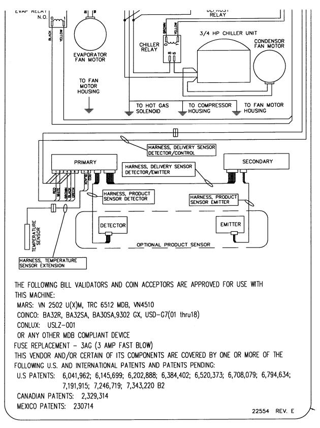
Figure 9.1 Typical Wiring Diagram, Sheet 4 of 4
