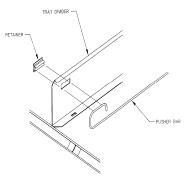
Figure 5.2 Pusher Bar Installation
