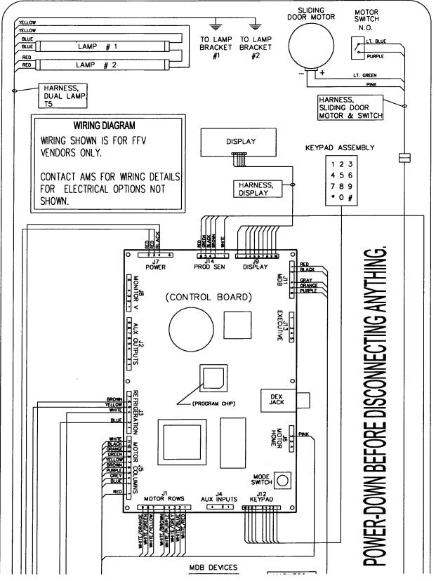
Figure 9.1 Typical Wiring Diagram, Sheet 1 of 4
