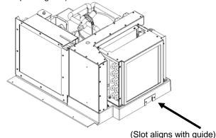
2. Insert the wedge tabs into the slots in the refrigeration base plate and in the slots in the cabinet.
