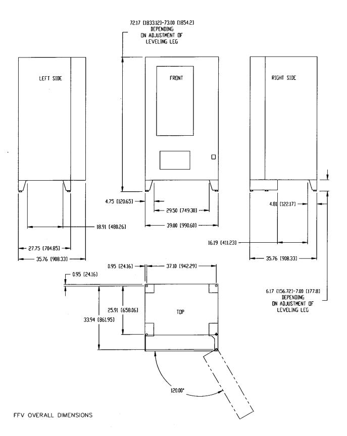
Figure 1.2 FV Cabinet Dimensions (For Reference Only)
