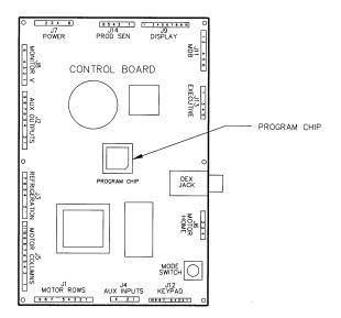
Figure 8.1 Replacing Program Chip
