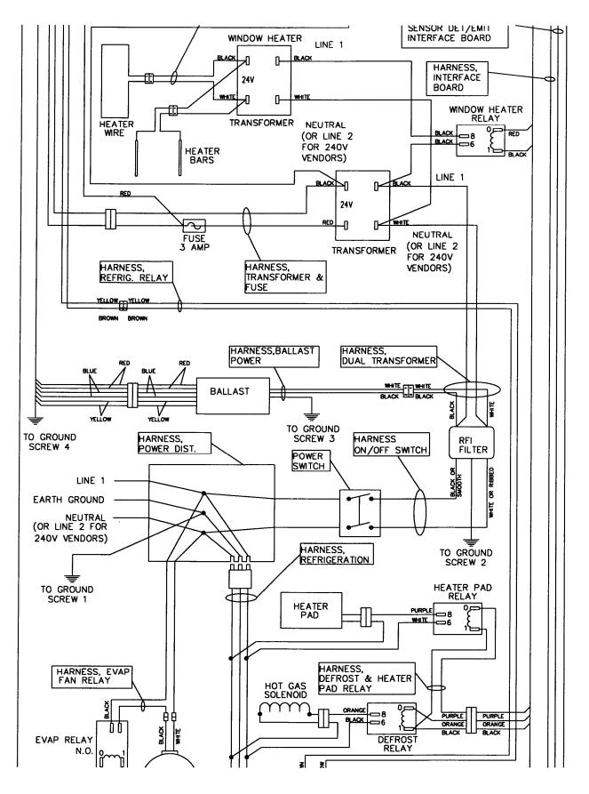
Figure 9.1 Typical Wiring Diagram, Sheet 3 of 4
