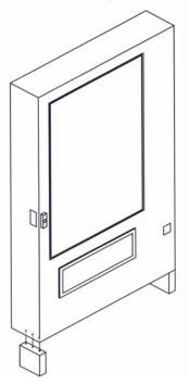
Figure 4.2 False Leg Installation
